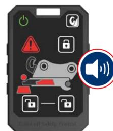
Quick coupler not correctly locked
