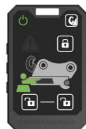
Quick coupler correctly locked
